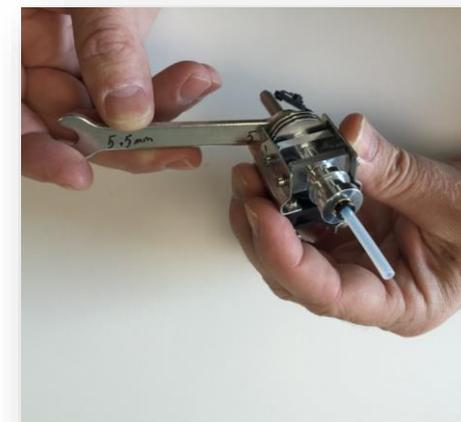
STEP 4. Install the heater block over the nozzle. Be sure the small set screws are unscrewed enough to allow the nozzle to pass through the heater block. Use the supplied 1.5mm hex wrench if necessary. **DO NOT FORCE THE HEATER BLOCK OVER THE NOZZLE!**
