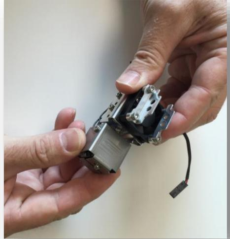
STEP 5. Tighten the heater block to the nozzles. **DO NOT OVER TIGHTEN THE SCREWS!** Only a small amount of tension is required to keep the heater block in place. Use the supplied 1.5mm hex wrench.
