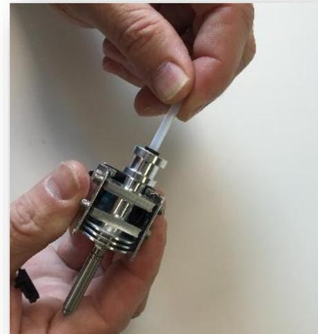
STEP 3 Tighten the nozzles. As you will see this forces the tube upward and tightens the tube into the fitting on top of the heat sink. It also seats the tubing deep into the nozzle. Your HYBRID will not work properly unless you follow this step.
