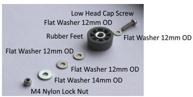
**STEP 2.1)** Place a Flat Washer 12mm OD onto a Low Head Cap Screw, then push this assembly through the underside of the Rubber Feet.
