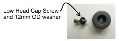
STEP 2.2) Then, place the two 12mm OD flat washers on the Screw.
