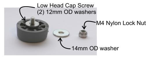
**Step 2.3)** Insert this assembly through one of the four corner holes of the printer. Then, from inside the printer, place a 14mm OD Flat Washer over the Low Head Cap Screw and attach an M4 Nylon Lock Nut. Repeat this installation process for all four corner holes. Use the wrench and nut driver to tighten. To assist with holding the nut, you can apply a little tape to the 7mm Nut Driver as shown.
