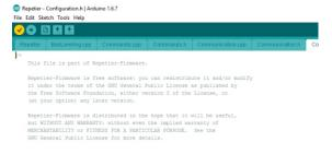
**STEP 8: Upload Firmware:** Click on the → to begin uploading the firmware to your printer. While the computer uploads the firmware to your printer, do not disconnect power to either the printer or the computer. If the firmware uploads successfully, it will give an "upload done" message. If the upload fails, repeat steps 7 and 8 again. Be sure to call or email us immediately if you are unable to upload the firmware.
