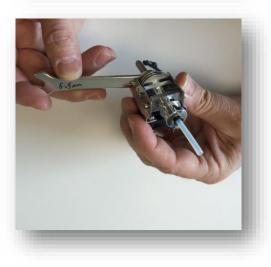
STEP 4. Install the heater block over the nozzle. Be sure the small set screws are unscrewed enough to allow the nozzle to pass through the heater block. Use the supplied 1.5mm hex wrench if necessary. **DO NOT FORCE THE HEATER BLOCK OVER THE NOZZLE!**
