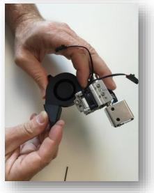
STEP 8. Rock the duct into position until it fits.
