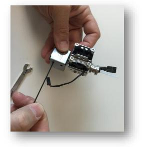
STEP 6. Installation of the blower fan is optional. For some filaments, such as PLA, the use of the blower fan is essential. For other materials, the blower fan can cause weak layer bonding. Use the supplied bolt and nut. You will need a 3mm hex wrench and 7mm wrench or socket. Use the upper holes, as shown!
