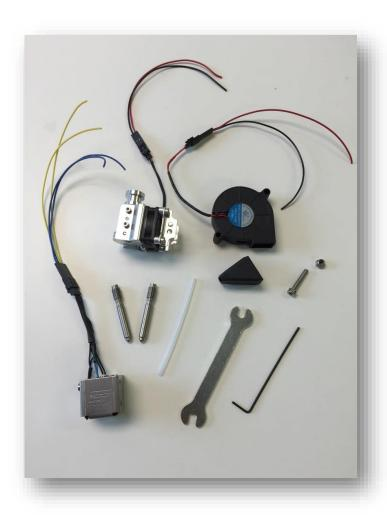
Heater block assembly, which includes a 100k Semitec 104GT2
